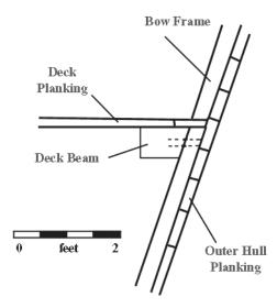
Figure 29. Deck / bow ramp interface.
