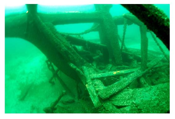
Figure 26. Port side bow. Note gentle curve of stempost and remnant of cross-planking just below knighthead. Photo by Tamara Thomsen.
