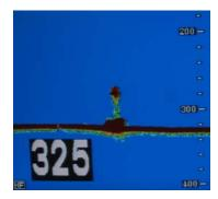
Figure 37. Sonar image of *Tennie* and *Laura* showing standing mast.
